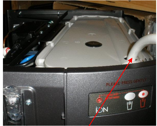
Siphon tube inserted to drain Ice Bank
