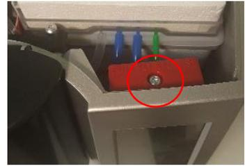
Lift tab on touch screen lock to unlock and remove
